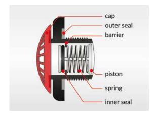
In a case tube was not used for longer time period, it is recommended to check functioning of all overpressure valves by pushing the spring with a finger or blowing through the valve. Parallely, seats of all valves shall be checked to avoid sand grains or dirt to block closing the valve.
